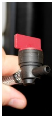
Tank valve closed
